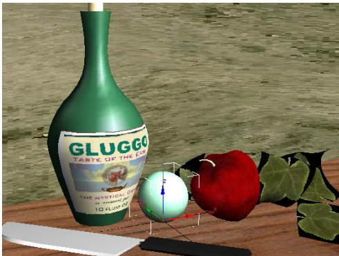
Create a sphere using AutoGrid
